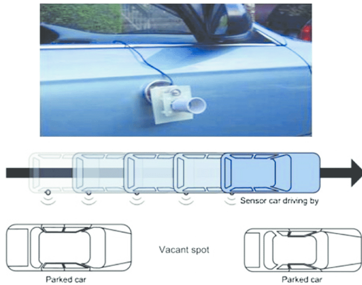
Figure 4.6.: The ultrasonic sensor mounted sideways on cars in the ParkNet system [59]
