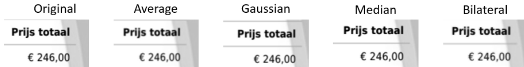
Figure 24: Zoomed in part of the image after blurring. The examples of the blurring techniques are tested on a digitally made invoice. The first figure shows the original image. The second figure shows the image after Average blurring. The second figure shows the image after Average blurring. The third figure shows the image after Gaussian blurring. The fourth figure shows the image after Median blurring. The fifth figure shows the image after Bilateral filtering. All techniques are realised with the OpenCV library.
