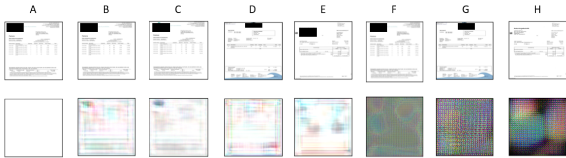
Figure 38: Different CAE results. A (2 different experiments): model 1 and 2 with loss MAE and optimiser Adam. B: architecture 1 MSE Adam 100 epochs. C: architecture 1 MSE Adam 200. D: architecture 1 MSE SGD 200. E: architecture 2 MSE Adam 200 (only transpose). F: architecture 2 (transpose+deconv) MSE Adam 50. G: architecture 2 (transpose+deconv) MSE Adam 200. H: architecture 2 (transpose+deconv) MSE Adam 200. All losses are very close 0, most of them are in the range of 0.500 to 0.000.
